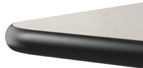
1300 / 1307 Bumper T-Mold 1-1/4" laminate top. The edges are banded with solid vinyl "T" molding, with 7/8" radius at corners. Modesty edge 1300
