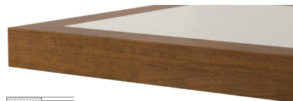
13500 1.25" fluted vinyl edge. High pressure laminate top standard with 3" radius corners. Available in a variety of colors
